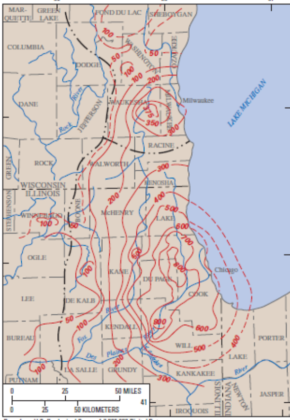
Base from U.S. Geological Survey 1:2,000,000 Digital Data Albers Equal-area Conic projection Standard parallels 33° and 45°, central meridian -89° EXPLANATION --- 700 --- Line of equal water-level decline, 1864-1980—Dashed where approximate. Interval, in feet, is variable - · - - - Major ground-water divide
