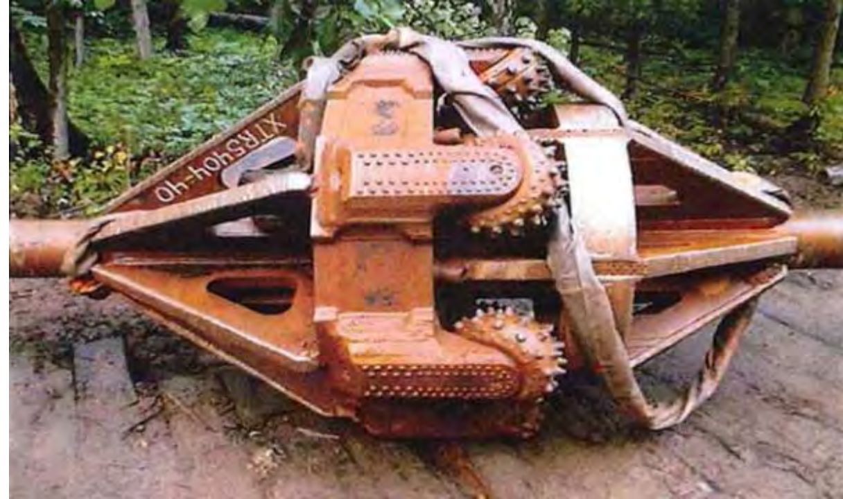
54 inch reamer similar to one lost during an HDD in New Jersey
