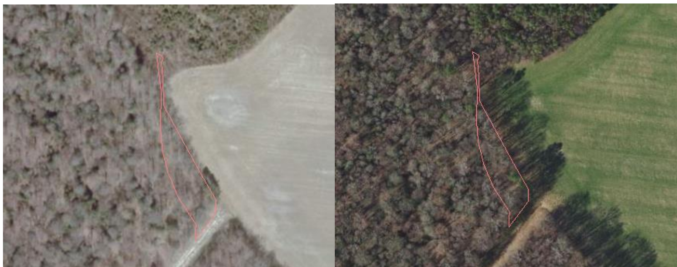
Map 2. An example of a polygon (outlined in pink) that was not altered between 2007 (left) and 2017 (right) but was included in the trends layer as a 'loss' because of computer mapping technique changes. Such cases are not included in loss calculations.
