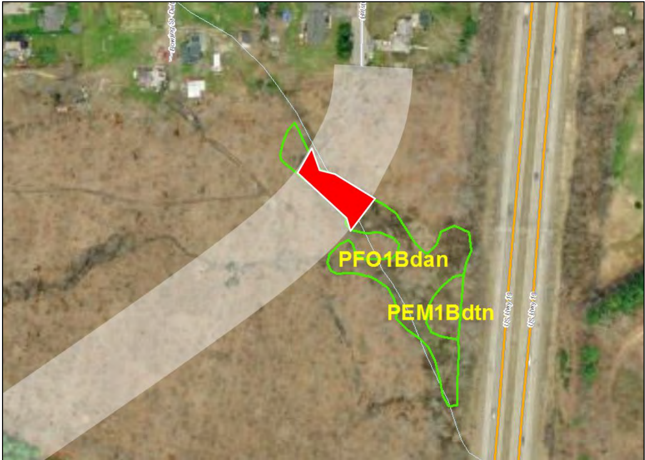
Wetland Unit with forested and emergent wetland types mapped in green, with yellow NWI codes. The white band represents the project area, which directly impacts 0.2 acres (shown in red) of the 1-acre AA (the Wetland Unit). In this case, a wetland delineation was available for the red project area, and the rest of the wetland was field-mapped with GPS.
